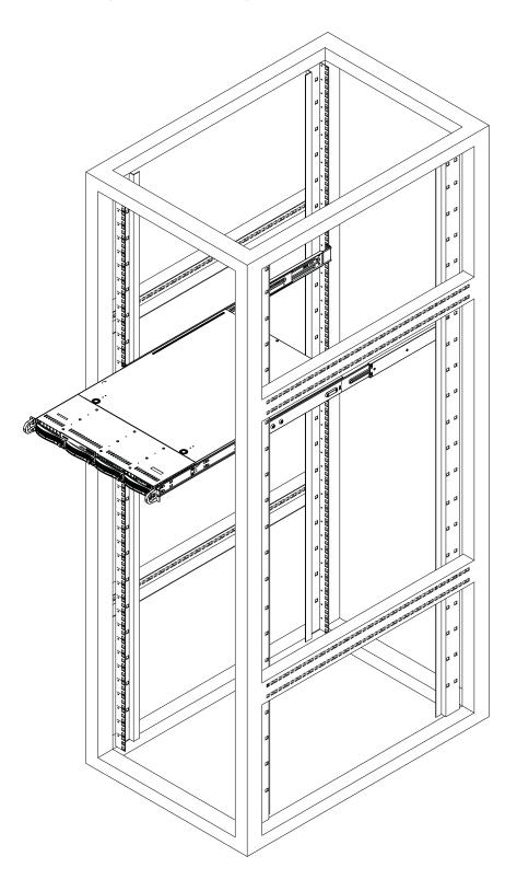
Figure 2-3. Installing the Server into a Rack
